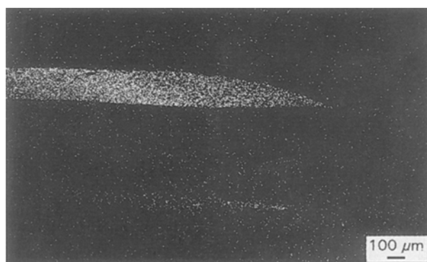
Figure 9 X-ray mapping of zinc near a weld nugget.
